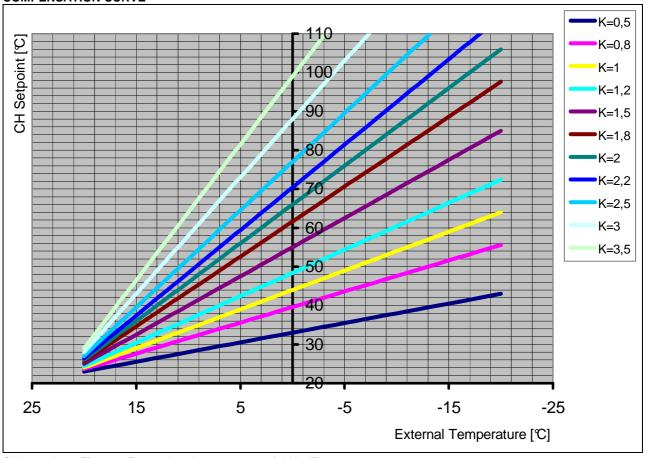
CH setpoint = (T<sub>ROOM</sub> – External probe temperature) \* K + T<sub>ROOM</sub>
