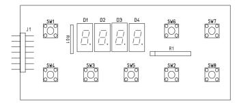
The control board is fitted with the following elements: 8 push-buttons (SW), enabling the user to carry out any adjustment and setting during installation; 4 displays (D1 ... D4) showing temperature, settings and failure codes. Two use modes are available: user's mode and installer's mode (by inserting a password).
