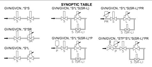
N.B.: The versions appearing in the Table of the connections and in the Synoptic table are available for any type of GVN/GVCN25, GVN/GVCN30 and GVN/GVCN40 and for any operating pressure.
