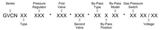
Series: GVCN = combined valve unit with connection
