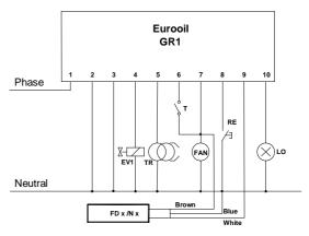
The following diagram instead shows an application example with a gas burner using an EUROGAS safety device type VM44G.
